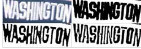
Figure 7.4: Impact of varying log-Gabor bandwidth for character segmentation. Original image (top left), binary version (top right), segmentation with large bandwidth (bottom left), segmentation with narrow bandwidth (bottom right).
