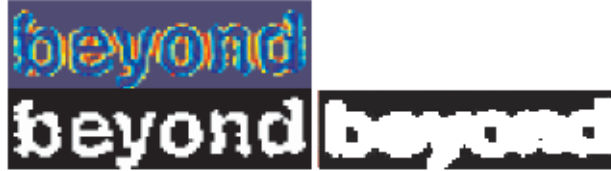
Figure 7.7: Phase of the vertical filter multiplied by the mask issued from the text extraction (top) and result after global thresholding (bottom left). Improvement is obvious from the binary version (bottom right).
