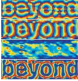
Figure 7.6: Log-Gabor filtering results for each filter property. From top to down: phase of the horizontal filter, phase of the vertical filter, magnitude of the vertical filter and absolute phase of the vertical filter.
