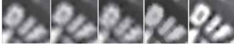
Figure 5.15: Comparison of SURETEXT and four best algorithms of the MDSP toolbox [98] for SR text. From left to right: ‘ Shift-And-Add ’ method (SA), Bilateral SA method, Median Gradient method with L_2 regularization, IBP with L_1 regularization and the SURETEXT result.
