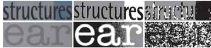
Figure 6.2: Segmentation conflict inside the RGBch color space. From left to right: original image, result inside RGB and result inside RGBch.
