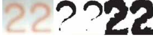
Figure 6.5: Example of failures of text extraction with RGB compared to HSV. From left to right: original image with varying colors and uneven lighting, extraction result inside RGB with k -means and extraction result inside HSV with k -means.
