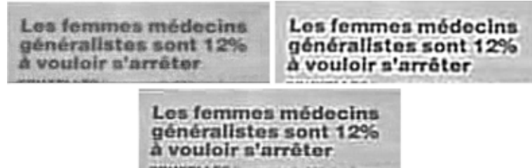
Figure 5.10: Results highlighting the importance of order of each step of SURETEXT. First row: left: classical approach ( med(S_1) ), right: Teager-filtered frames after median fusion with an interpolated original frame. Second row: the result from SURETEXT.
