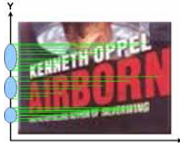
Figure 7.1: Illustration of line segmentation for skewed text: three clusters based on the y -coordinates of connected components.
