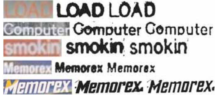
Figure 7.9: More character segmentation examples. From left to right: original image, SMC-based binary version and result after character segmentation.
