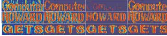
Figure 6.13: Same examples of Figure 6.11. From left to right: result of the absolute phase of the vertical log-Gabor filtering, after applying mask obtained by D_{eucl} -based extraction, after applying mask obtained by S_{cos} -based extraction and after applying mask obtained by global thresholding. More explanations about the use of log-Gabor filtering are given in Chapter 7.
