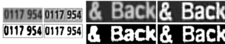
Figure 5.12: Two zoomed in SR results comparing the classical approach (on left of each result) and the proposed method (on right of each result) and their binarized images (bottom row).
